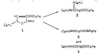
amine reacts slowly with 1 at room temperature in  $CCl_4$ ,  $CH_3CN$ , or 95:5  $Me_2SO/H_2O$  to form amidine 2. However, when  $60:40 \text{ CH}_3\text{CN}/\text{H}_2\text{O}$  was used as a solvent, a rapid reaction led to the formation of a mixture of diamide 3 and malonamate 4. The latter undoubtedly resulted from the base-catalyzed reaction of water with 1 accompanied by loss of  $CO_2$ .
